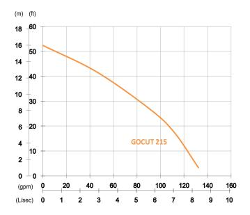
Shaft Speed: 2850 rpm Outlet: 50mm, 2in
